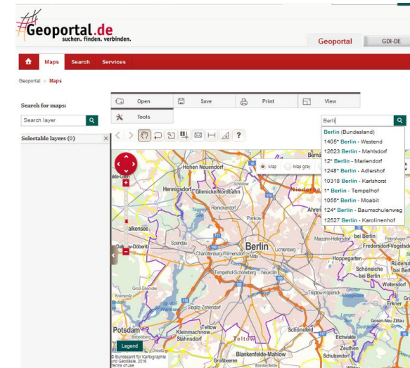
Figure 16-1 The German national geographical names database (GN-DE) published as a web service as part of the national spatial data infrastructure (GDI-DE) and visualized through the Geoportal application (Geoportal.de)
